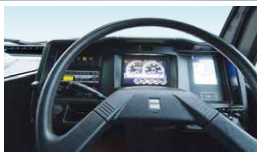
▲Equipped with a LCD cluster meter and a touch screen information display
