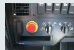
▲Mobile phone storage & Pedal operation selector switch
