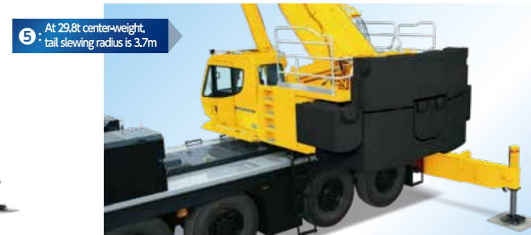
3 At 21.8t center-weight, tail slewing radius is 3.7m
